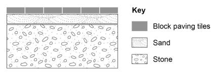
To build block paving
