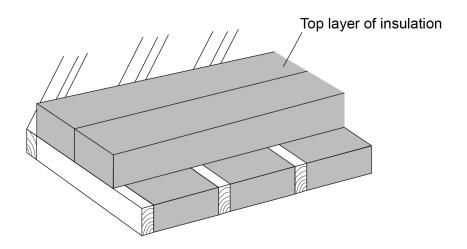
Use the full area of the loft to work out how many rolls of top layer insulation you need.
