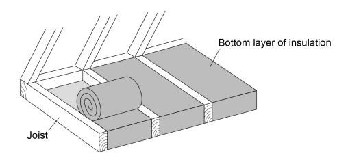
Subtract 10% from the area of the loft to allow for the joists.
