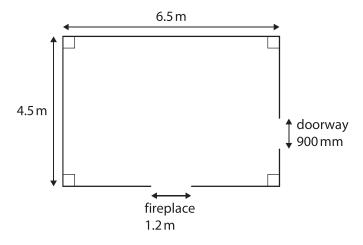
Skirting boards come in lengths of 2.4 m The lengths of skirting board can be cut and joined.
